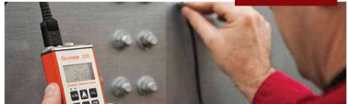
NDT for Shell gauging of LPG tanks
